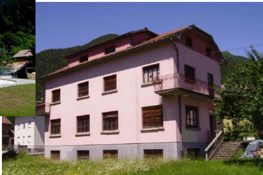
*Comune di Paluzza (UD) 3297 GG –  $S_{Netta}=282$  mq –  $S/V=0,63$  –  $PT_{Risc}=8,7KW$  –  $IE=21$  kWh/m<sup>2</sup>a*
